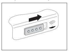
Slide the ON/OFF switch for the radio components in the direction of the arrow to start the LaunchManager.
